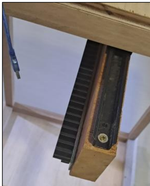
Fig. 11: How this system used the drawer slides of the cupboard drawer holder system
