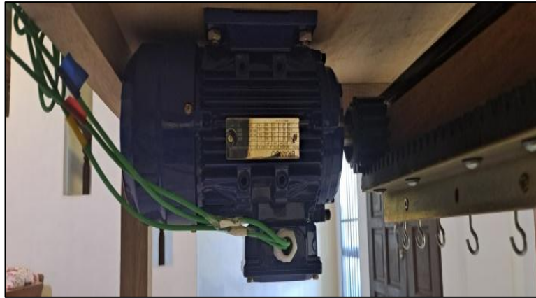
Fig. 10: The gear attached to the induction motor turning the toothed rail which will hold the clothes
