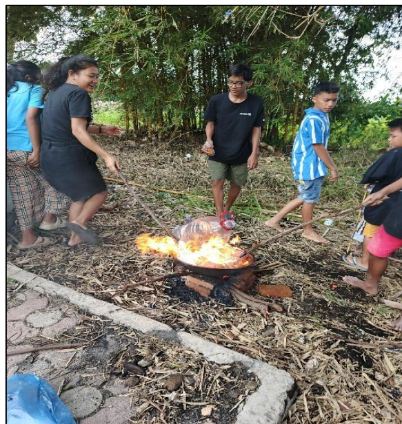
Figure 6. BKM children are melting plastic waste to be used as the main material for paving blocks (Source: personal document, 2025)
